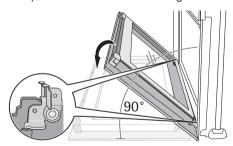
2. Loosen the **clamp levers** on both door hinges (A) **completely** .
